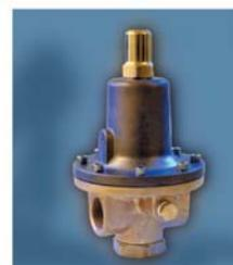
REGO's BR-1780 series regulators are specifically designed for final-line pressure regulation for hospital oxygen systems. Equally suitable for variety of gases in medical or industrial applications. Balanced seat design provides constant delivery pressure ranges (5-55psig, 40-110psig, 100-200psig) with varying inlet pressures (up to 400 psig) and wide range of flow demand. Temperature range -40°F to 165°F. Flow rates up to 16,000 SCFH.
